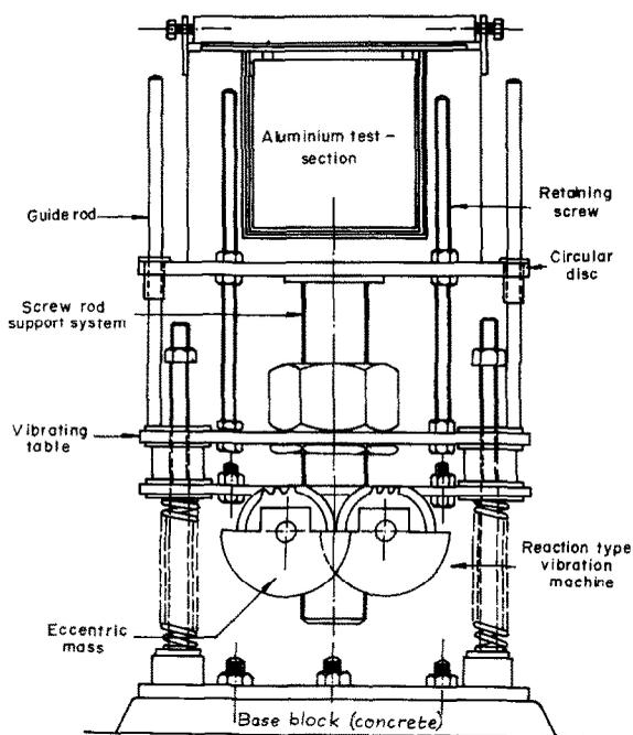
FIG. 2. Details of test section and vibration machine assembly.
