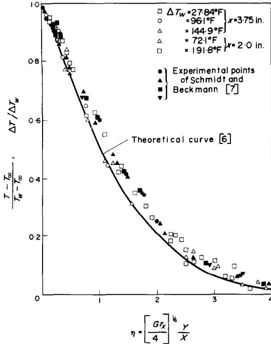
FIG. 3. The free convection temperature profile.
