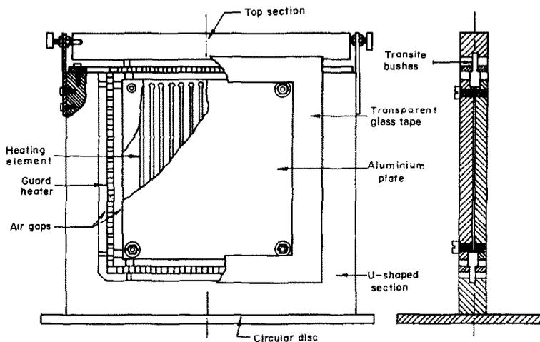
FIG. 1. Construction of test plate.
