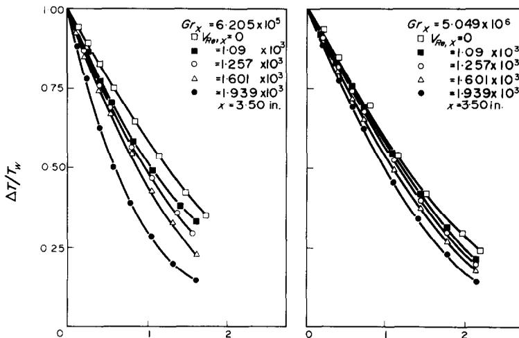
FIG. 4. Effect of  $V_{Re,x}$  on temperature profiles at  $Gr_x = 6.205 \times 10^5$  and  $Gr_x = 5.049 \times 10^6$ .
