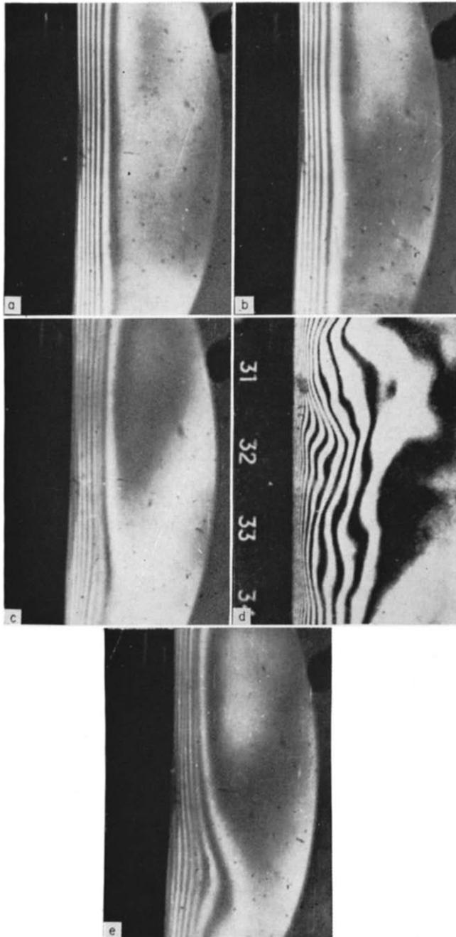
FIG. 7. Zero-fringe interferograms of the boundary layer under oscillating plate conditions
